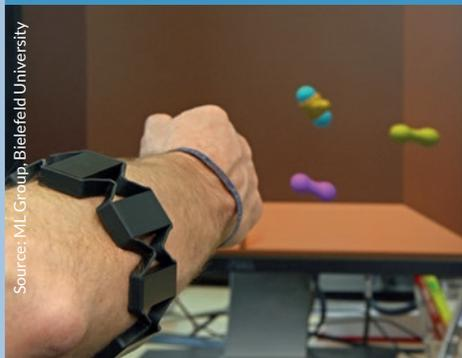
*Transfer learning technologies developed at Bielefeld University enable a rapid recalibration of cuff electrodes for hand prosthesis*
